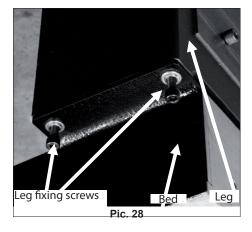
Lay the bed on timbers in the upside down position. Lift the legs to the vertical position and lower them onto the bed. Secure with the fixing screws provided.
